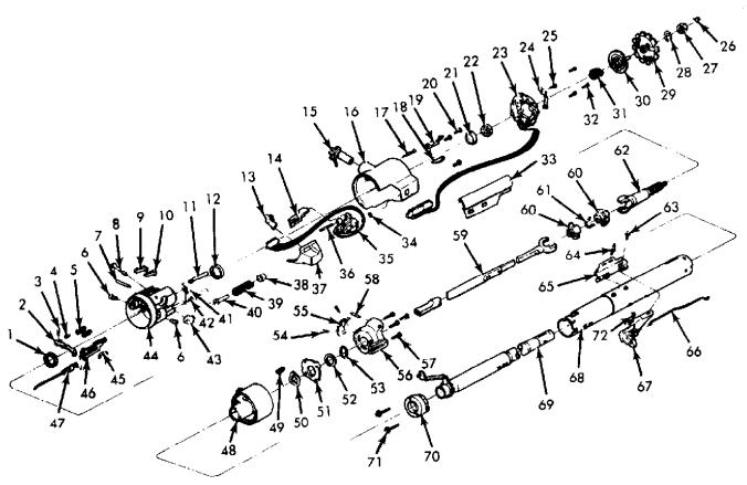
Bearing Assembly 2. Shoe Release Leve 3. Release Lever Pin Shoe Release Lever Release Lever Spring 5. Shoe Spring 6. Pivot Pin Dowel Pin 8. Drive Shaft 9. Steering Lock Shoe 10. Steering Lock Shoe 11. Lock Bolt 12. Bearing Assembly 13. Tilt Lever Opening Shield 14. Dimmer Switch Actuating Rod 15. Lock Cylinder Set16. Lock Housing Cover17. Lock Retaining Screw18. Buzzer Switch Retaining Clip19. Buzzer Switch 20. Screw 21. Inner Race 22. Upper Bearing Inner Race Seat 23. Turn Signal/Flasher Switch
