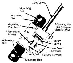
Fig. 9: Aligning Dimmer Switch
