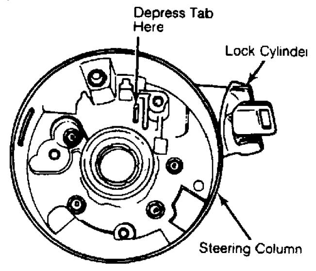
$\frac{2/902}{\text{Fig. 2: Removing Lock Cylinder}}$
