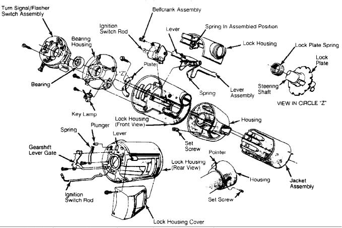
Fig. 5: Exploded View of Column Shift Steering Column Housing
