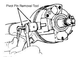
27112 Fig. 4: Removing Pivot Pin
